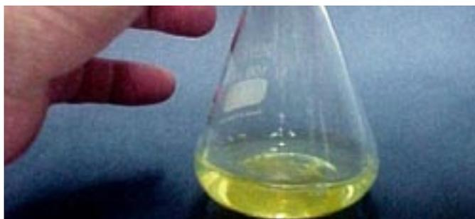
**Figure 1** Before the addition of any silver nitrate the chromate indicator gives the clear solution a lemon-yellow colour.
