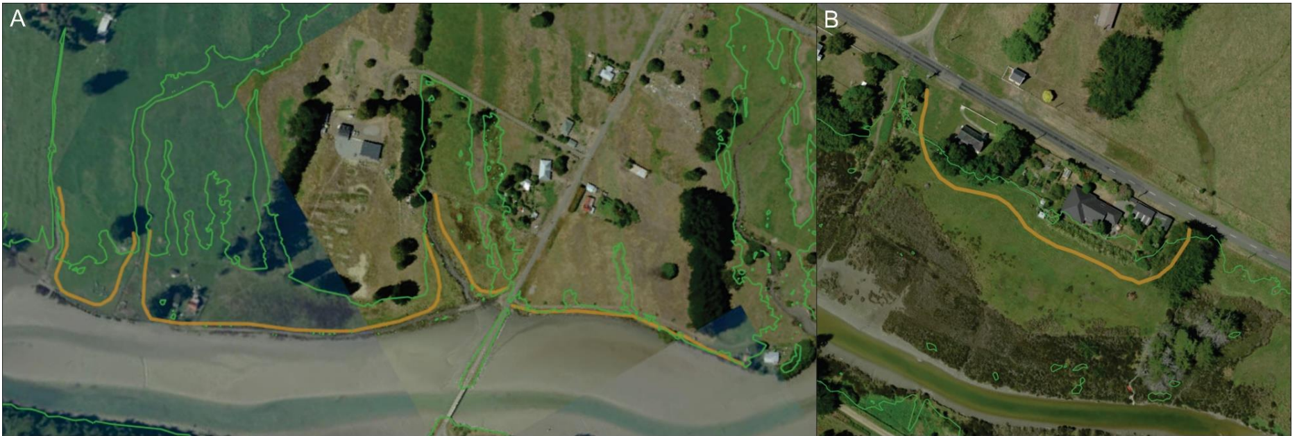
Figure 20: Proposal of inundation bunds to protect low lying assets and productive farmland. Localised protection provides by inundation bunds constructed from excavated sediment from drainage network. Inundation bunds depicted as orange lines extend from lower land areas to meet 1.5 m contour line, depicted as green lines. A) Areas at low lying levels proximal to Churlton Road Bridge. B) Low lying areas of St John the Evangelist Church and the Vicarage.
