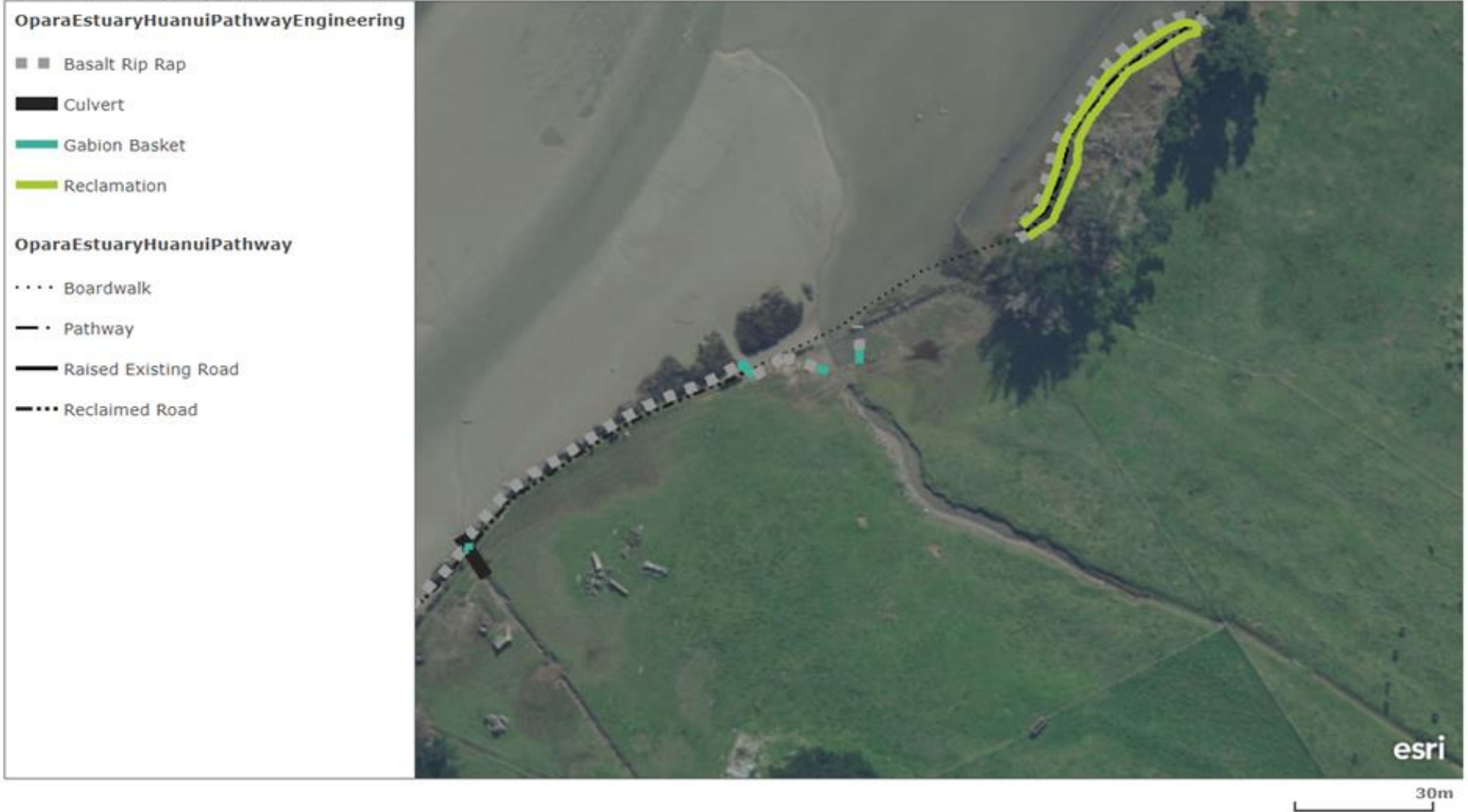
Figure 19: Opapa Estuary Huanui Pathway close-up highlighting the locations of basalt rip rap, culverts, gabion basket, reclamation, boardwalk, pathway, raised existing and reclaimed paper road.
