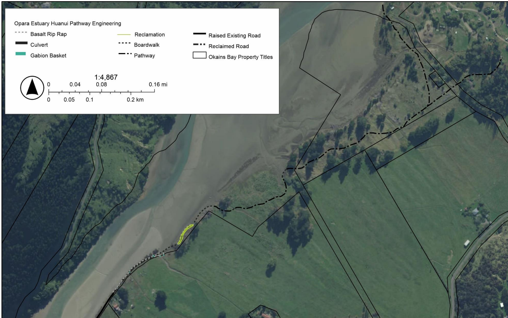
Figure 18. Opara Estuary Huanui Pathway with suggested basalt rip rap, culvert, gabion basket, reclamation, boardwalk, pathway, raised existing and reclaimed road.
